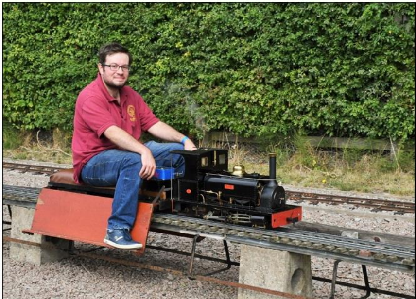
George Winsall (Rugby MES) with his 3½ in. gauge Hunslet 0-4-0T Lilla built to Don Young's drawings.
